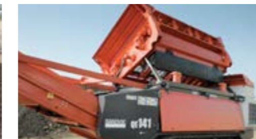
Tipping function activated by radio remote control
