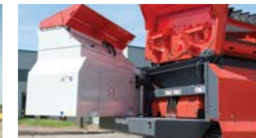
Hydraulically opening powerpack for ease of maintenance
