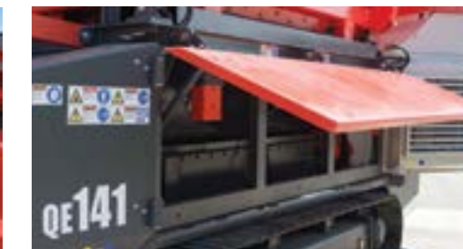
Hydraulically folding doors for easy access
